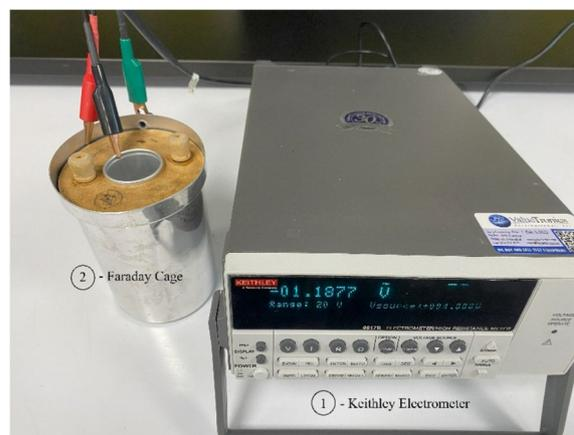
**Fig. 1** Charge measurement with Keithley 6517B electrometer (1) and Faraday cage (2)
