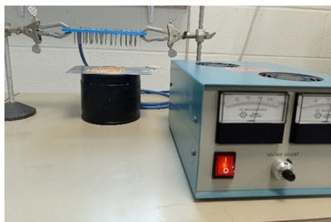
**Fig. 2** Corona charging of plant biomass
